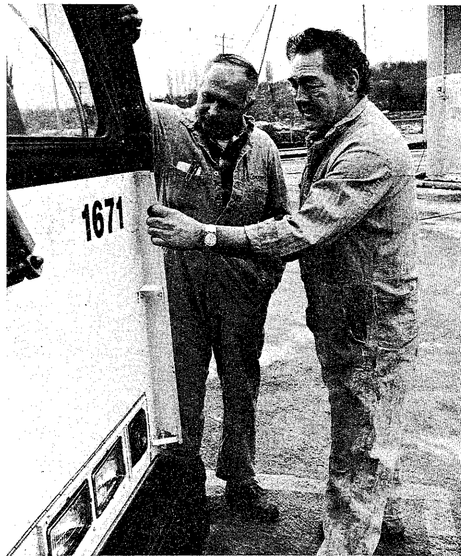
George Tague (left) and Al Blanes, automotive sheet metal workers, inspect a prototype wind-deflector that keeps mud and spray away from the rear-view mirrors and side windows of 1600-series buses.
