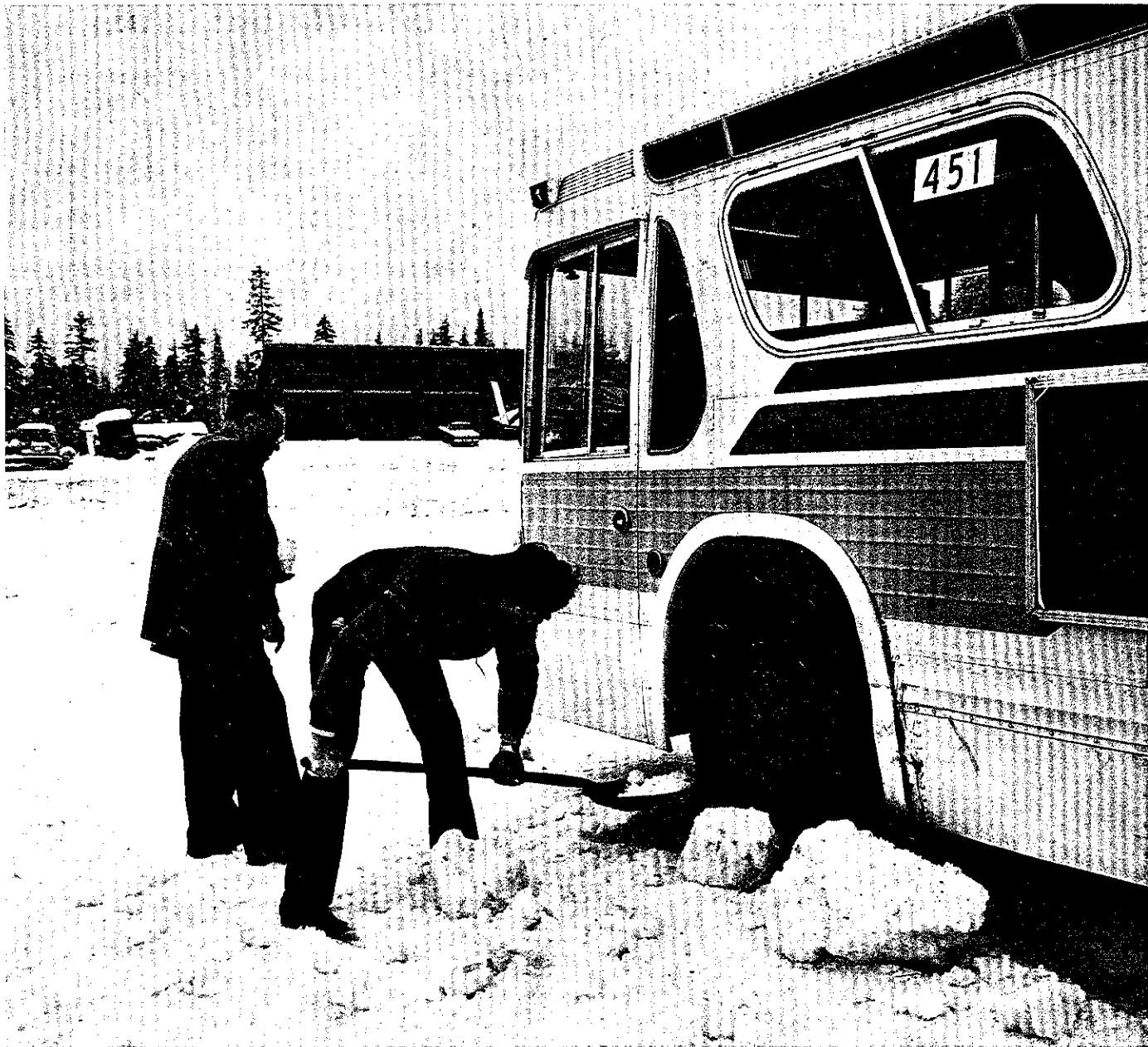
At Snoqualmie Pass Scan Manufacturing factory representative Russel Bryant, right, packs snow in front of a Metro bus to test how an automatic snow chain system
