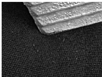
The tip of the wheel block blown up from the photo above; please note that the seat pan has a bowl shaped contour but the "padding" doesn't yield to the weight of the wheel block.
