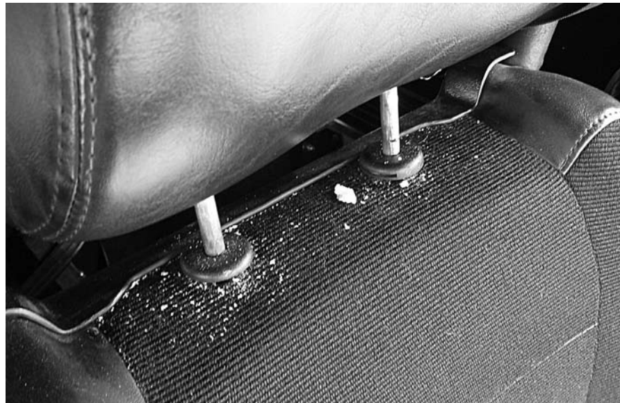
Ever wonder what the "cracker crumbs" are on the top of our seat backs? It is the headrest foam becoming brittle and falling out.
