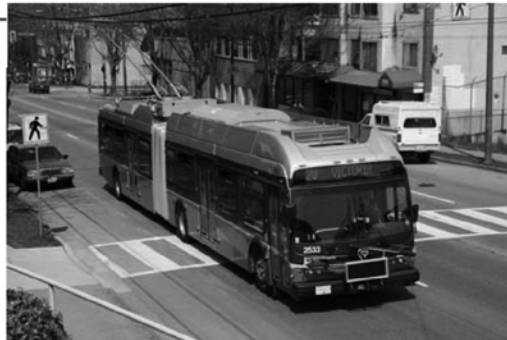
Electric trolley buses, such as this one in Vancouver, B.C., draw electricity from overhead wires.
