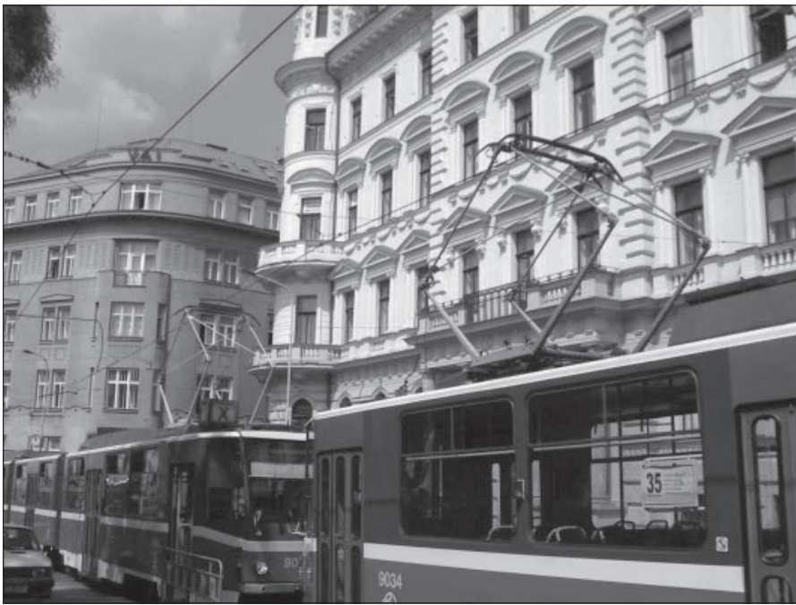
Trams in position to go. Note the single overhead contact. The vehicles are grounded in the steel rails.
