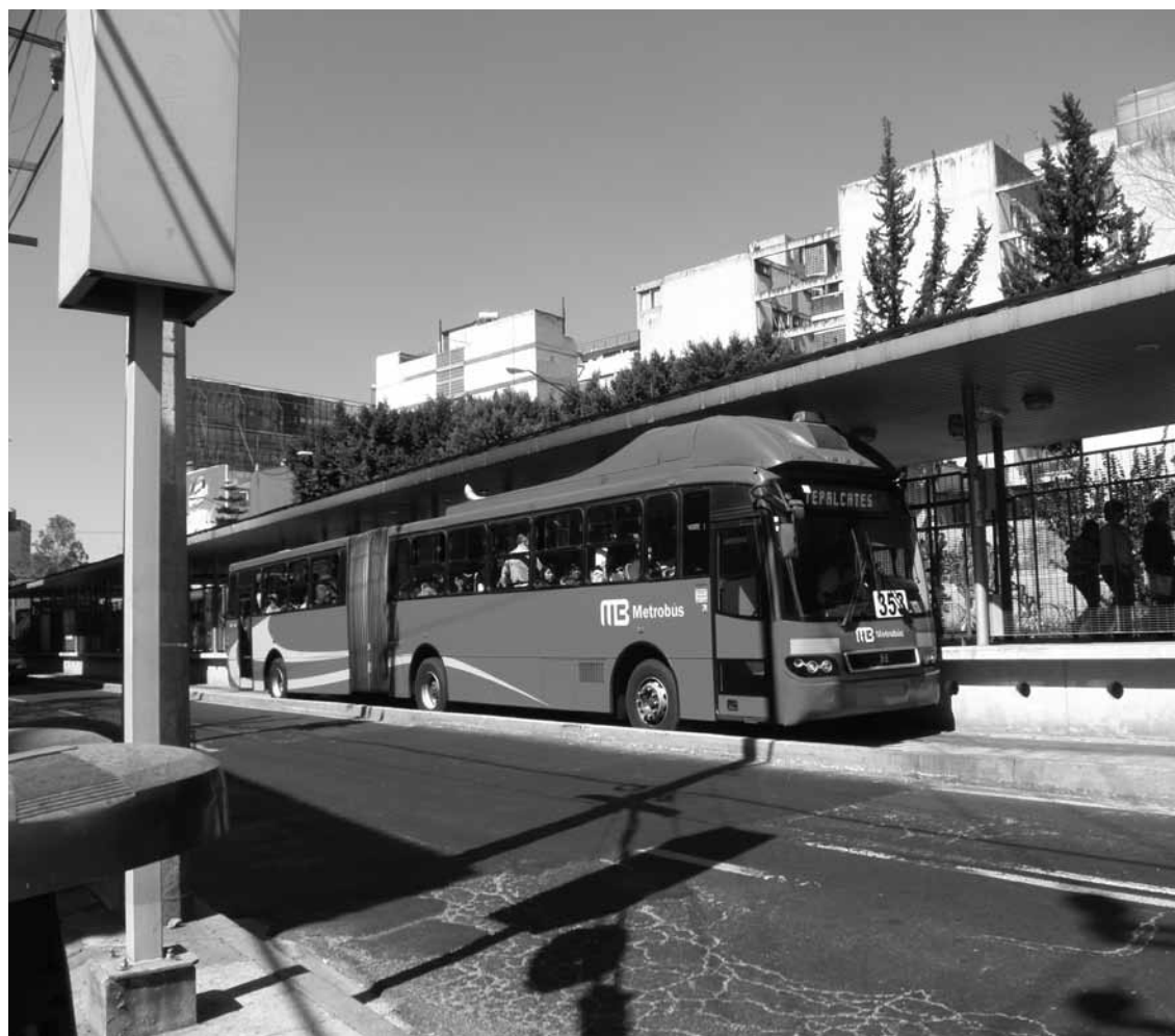
A bus pulling into a station. The doors visible on the right side of the bus are for emergency purposes only.
